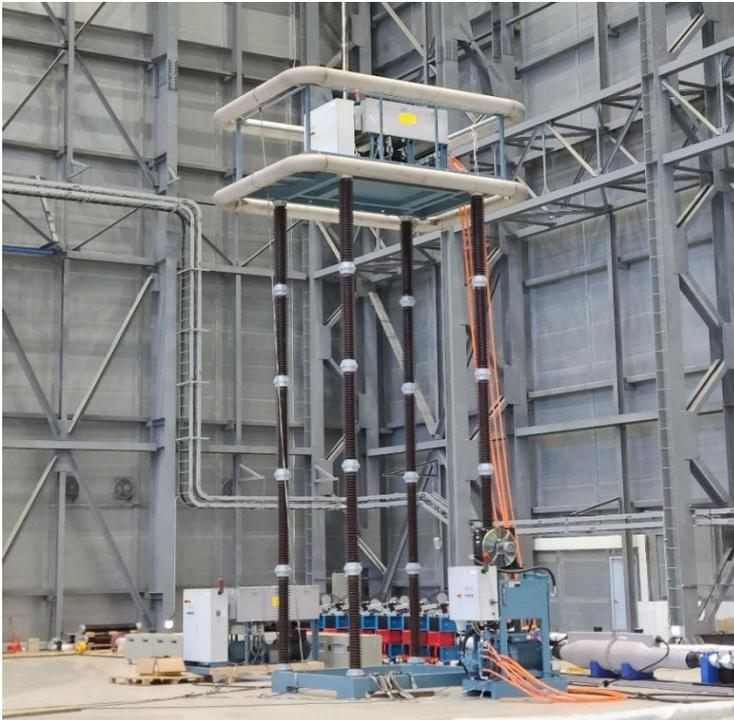
Test Loop Current Source
